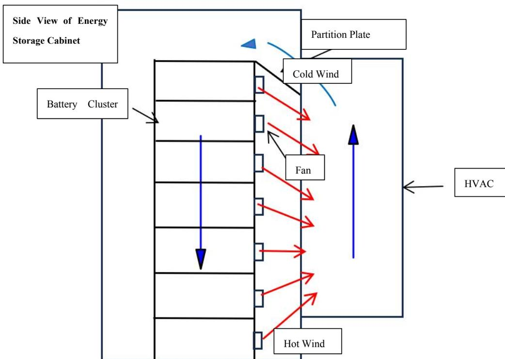
**System Cooling Layout Plan**
