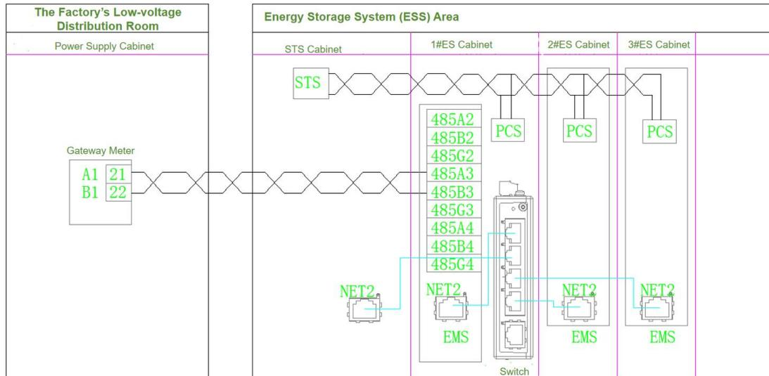
**Cabinet communication interface diagram of industrial and commercial off-grid energy storage system**
