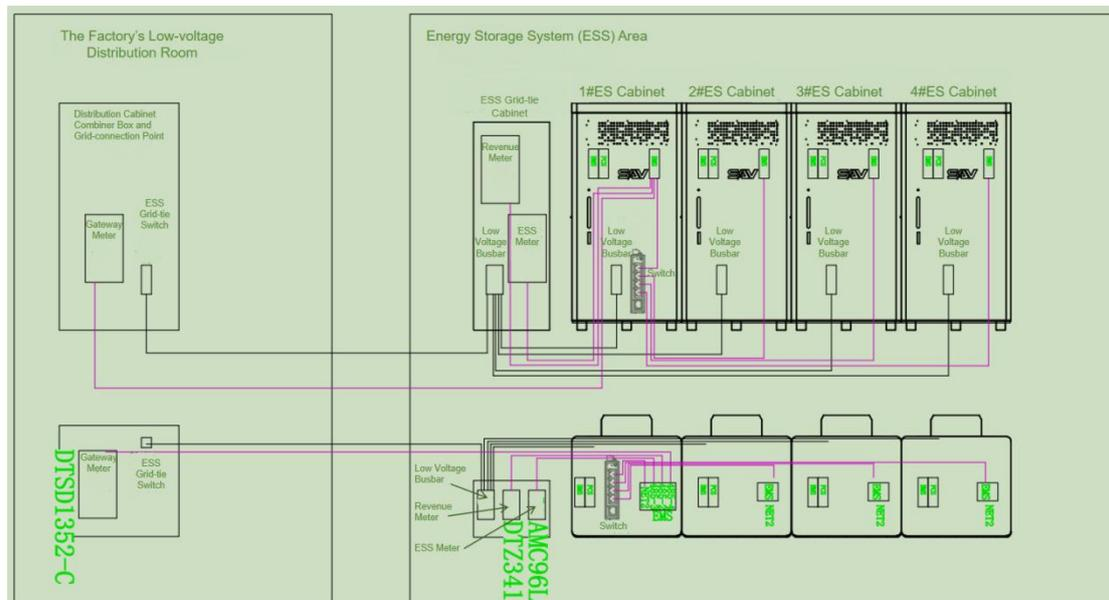
**Cabinet wiring diagram of industrial and commercial grid-connected energy**
