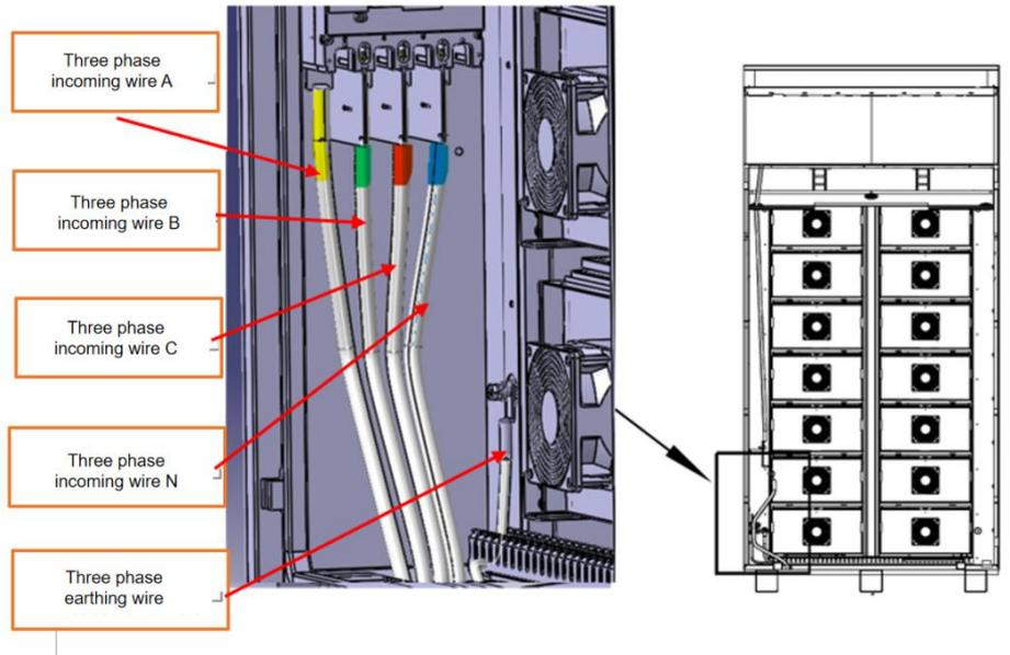
**Single cabinet wiring diagram in an industrial and commercial grid-connected energy storage system**
