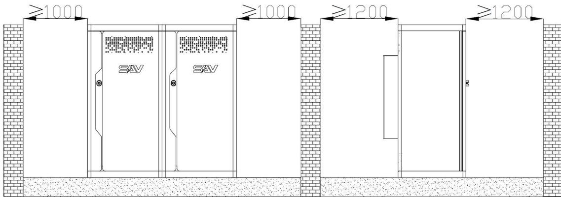
**When installing multiple cabinets, the space requirements are as follows:**
